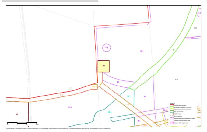
Site 43 is a relatively small rectangular area of approx. 0.36ha. northwest of Longbarrow Roundabout. The site lies within the Main Civils Compound site and is required for the construction of a temporary electricity substation and water supply connection.
